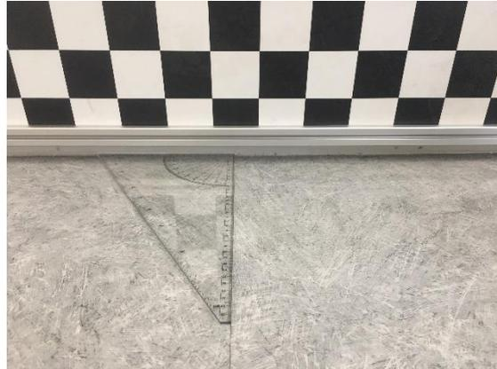
*Finding a line perpendicular to the wall*
