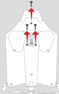
7 Use a PH2 screwdriver to remove the 3 screws holding the C.H.U.C.K. under the Parrot Disco.
