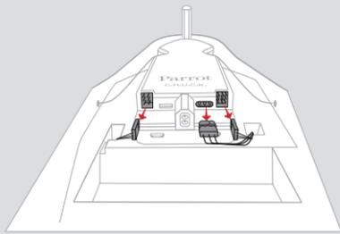
5 Unplug the servomotors and the motor of the Parrot Disco.
