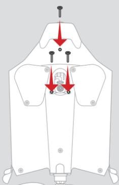
2 Use a PH2 screwdriver to secure the C.H.U.C.K.
