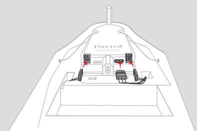
4 Connect the servomotors and the motors back to the C.H.U.C.K.
