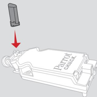
2 Put the new pitot tube into place.
