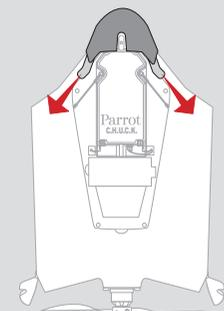
8 Once the nose is in place, remove the four protections and press on the new nose to make it stick properly to the EPP.
