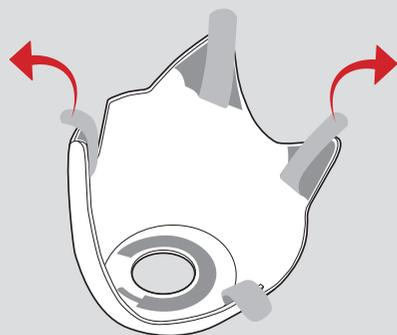
5 On the new nose, fold the four protections towards the outside of the blister.
