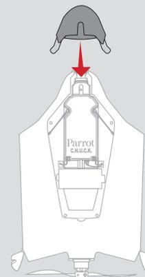
7 Slide the new nose in place. Make sure the four left protections are sticking out.
