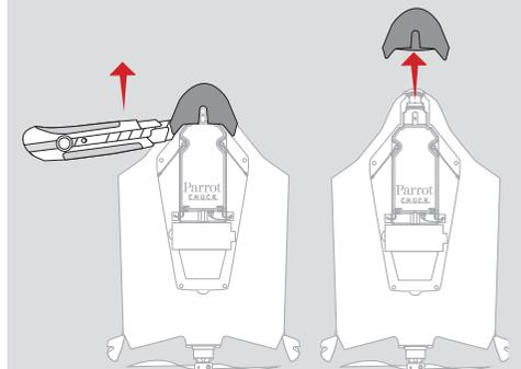
4 Using a box cutter, gently remove the nose of the Parrot Disco.
